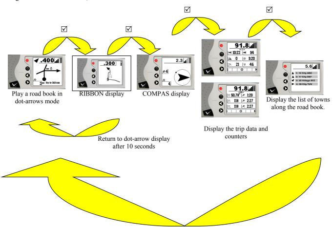
The «RIBBON» display is automatically activated when approaching the starting point of a selected roadbook (when within 400 m (0,25 mile) from the starting point). It is also automatically activated when approaching the itinerary when the vehicle was previously off-route (in compas mode). The «RIBBON» display is also permanently displayed when riding an itinerary in the opposite direction to the one selected.
